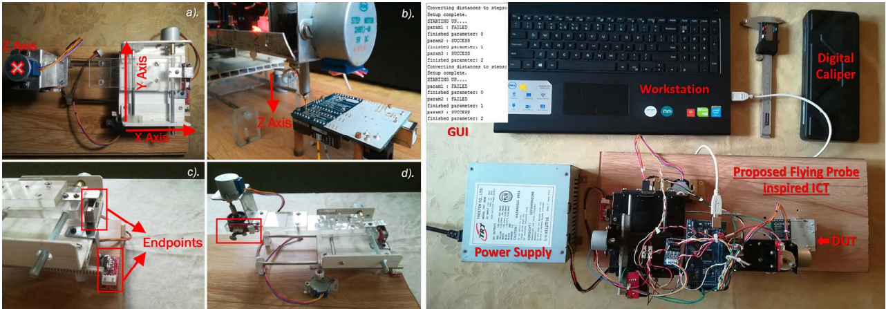
Fig. 1. Left: FPICIT Mechanical Structure with Axis Array (a, b) and Mechanical Endstop Limit Switch (MELS) Placement (c, d). Right: Complete experimental setup for the proposed FPICIT.
